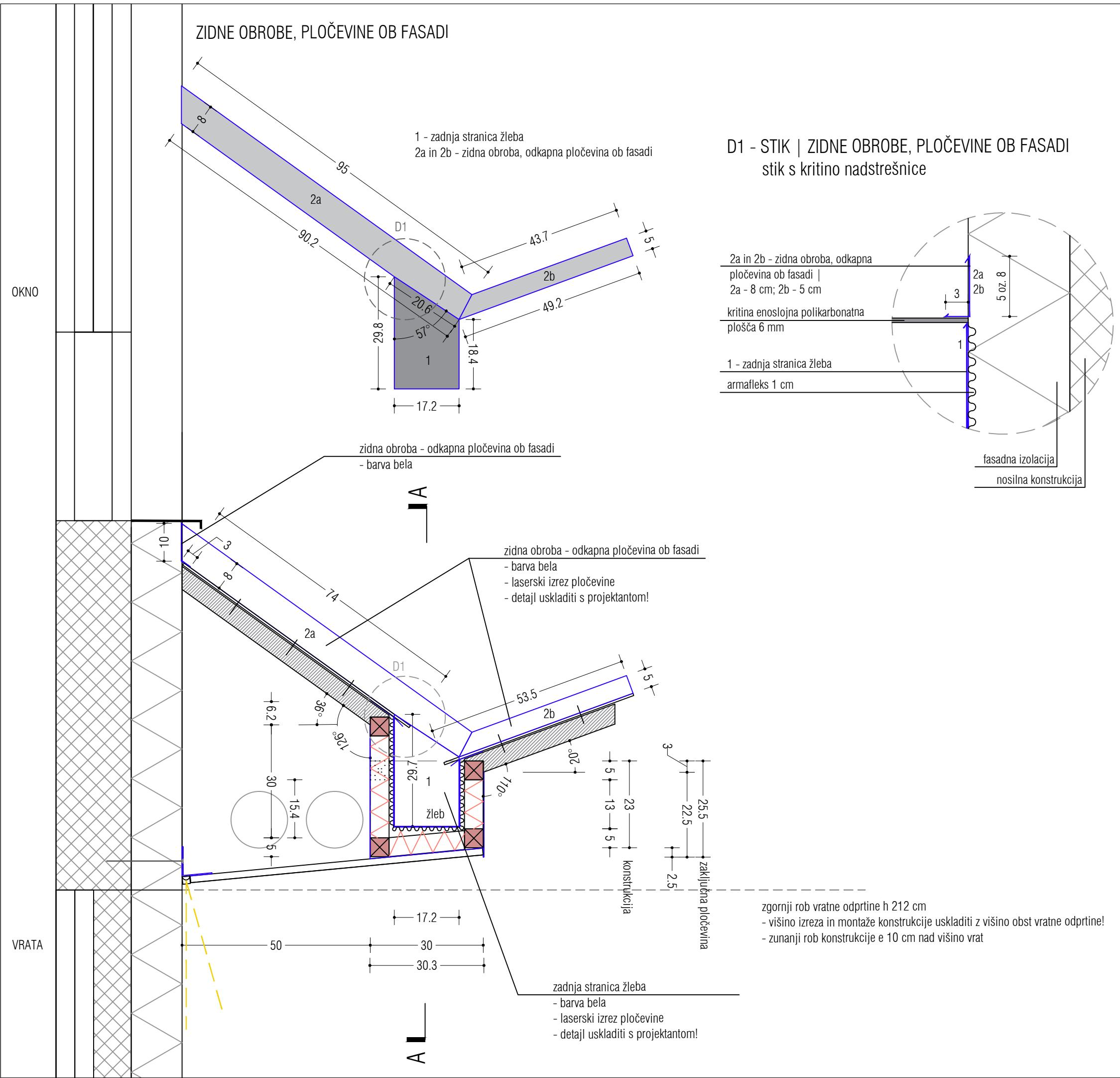
D2 - ZAPIRANJE KONSTRUKCIJE NA OBST. AB ZIDU
